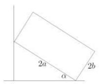
The diagram shows a uniform rectangular lamina with sides of lengths 2a and 2b leaning against a rough vertical wall, with one corner resting on a rough horizontal plane. The plane of the lamina is vertical and perpendicular to the wall, and one edge makes an angle of  $\alpha$  with the horizontal plane. Show that the centre of mass of the lamina is a distance  $a\cos\alpha + b\sin\alpha$  from the wall.
